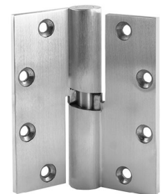
■ A9500 Cam Lift Hinge 5" x 4.5" Cam Lift Hinge 5/16" of lift, can hold up to 900lbs.
