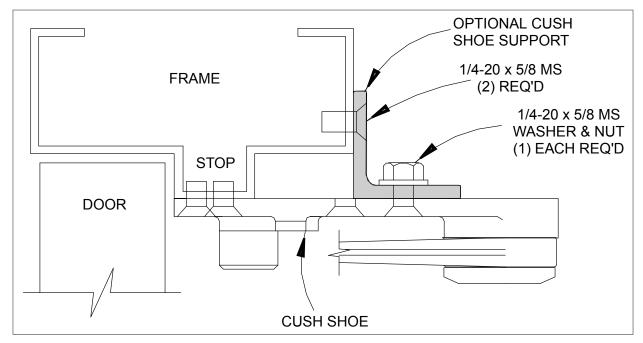
Should frames have 1/2" Blade Stop it is necessary to use 1/2" Blade stop Spacer (available from Dealer). Use both Blade Stop Spacer and Shoe Support wherever required.
