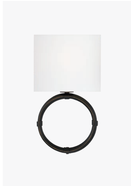
▲ 645211IH OGDEN SCONCE Brushed Black Iron 8"W x 14.5"H x 6"E Backplate: 7.5"W x 6.75"H x 0.75"E Ctr/top: 3.25" Ctr/btm: 11.25" 1 - 60 Watt E12 Candelabra White Fabric Bolt-On Shade Damp Rated
