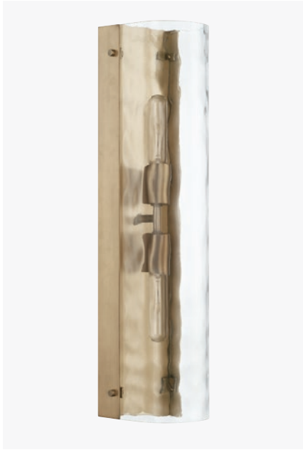
▲ 627521AD LYRA SCONCE Aged Brass 5.5"W x 22.25"H x 5.5"E Backplate: 5"W x 22"H x 0.75"E Ctr/top: 11" Ctr/btm: 11" 2 - 100 Watt E26 Medium Clear Water Glass Damp Rated Vertical or Horizontal Orientation
