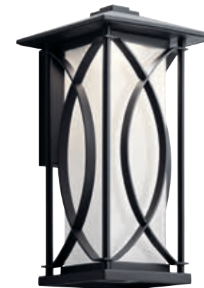
49974BKTLED | Outdoor Wall 7.5W, 3000K, 90 CRI, 40 LPW 8"W x 15"H | Ext. 8" W LED
