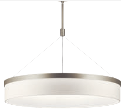
42298SNLED | Chandelier/Pendant 3Lt LED (3) 38W, 600lm, 3000K, 90 CRI, 16 LPW, 18.5"H x 26.5"W Overall Ht. 57.25", Chain/Stem 36"
