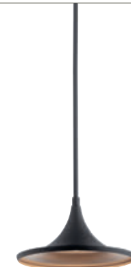
59030BKTLED | Elias (1) 9W, 425lm, 3000K, 90 CRI, 44 LPW 6"H x 11"W Overall Ht. 52.25"
