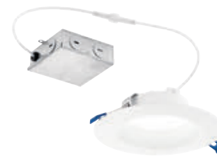
DLRC06R3090WHT Direct-to-Ceiling Recessed (1), 13W, 900lm, 3000K, 69 LPW 8"W x 2"H, | 0.16"H from Ceiling 22"L with cord+box W T24 LED
