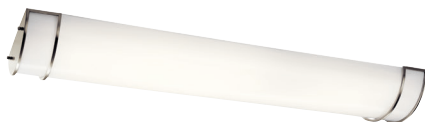
11304NILED Brushed Nickel | White Acrylic (1), 55W, 3400lm, 3000K, 90 CRI, 62 LPW 11.5"W x 4.75"H x 49.25"L D F T24 ADA Dimmable LED
