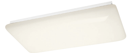
10303WHLED White | White Acrylic (1), 80W, 5725lm, 3000K, 90 CRI, 72 LPW 16.75"W x 5"H x 51.5"L D F T24 ADA Dimmable LED
