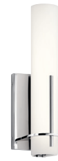
83944 | Traverso Chrome | Etched Opal Glass (1), 21W, 1100lm, 3000K, 91 CRI, 52 LPW 4.5"W x 13"H | Ext. 3.86" D LED
