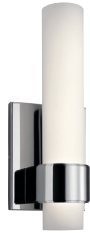
83745 | Izza Chrome | Etched Opal Glass (1), 21W, 850lm, 3000K, 91 CRI, 40 LPW 4.75"W x 13"H | Ext. 4.35" D LED
