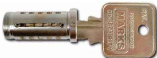
Plug with INCORRECT alignment (A visual test)
