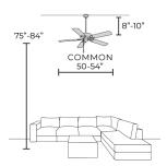
A fan should be 75-84" from the ground while keeping 36-48" above a seating area. For optimal air distribution keep 8-10" from the ceiling.
