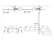
Large open spaces may require more than one fan in the room. Fans should be spaced 24-36" away from any wall, and leave at least 36-48" between fans.
