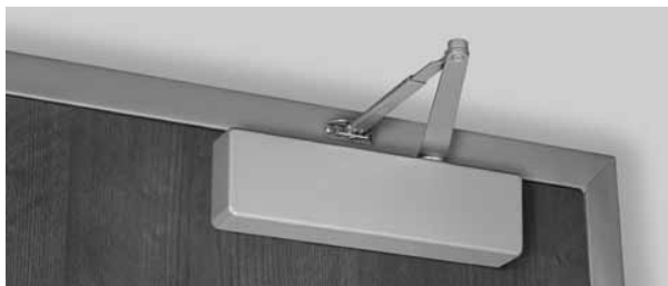
Regular Arm - allows closer to be installed where there is as little as 1" (25mm) of frame face or ceiling clearance.
