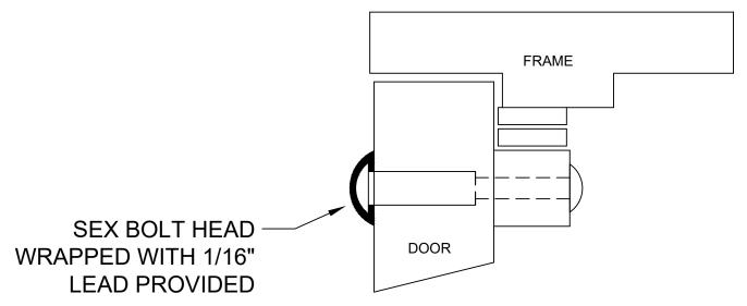
Sex bolt head comes wrapped with Lead. Bolt to be inserted into the thru-bolt prep in door per standard template.
