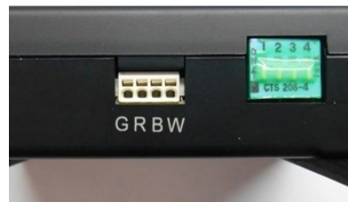
Figure 8: XT AIM 4-wire terminal for connecting power supply & DIP switch bank
