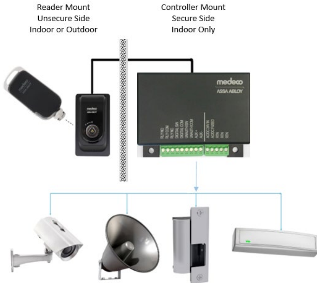
Figure 1: XT AIM Reader and Controller System
