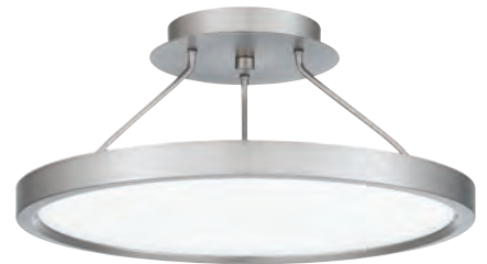
OST1815BN 6.75" H x 15" W x 15" D Finish: Brushed Nickel Integrated LED Lumens: Delivered 1890 | Initial 2700 Kelvin 3000, CRI 90 ETL Listed Location: Damp
