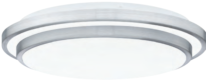
IVG1616BRA 3.25" H x 16" W x 16" D Integrated LED Lumens: Delivered 1525 | Initial 2500 Kelvin 3000, CRI 90 ETL Listed Location: Damp (NOT TO SCALE)
