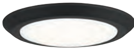
VRG1612EK 1.75" H x 12" W x 12" D Integrated LED Lumens: Delivered 1037 | Initial 1480 Kelvin 3000, CRI 90 ETL Listed Location: Damp
