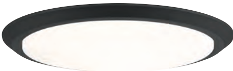
VRG1620EK 2" H x 20" W x 20" D Integrated LED Lumens: Delivered 2190 | Initial 2580 Kelvin 3000, CRI 90 ETL Listed Location: Damp
