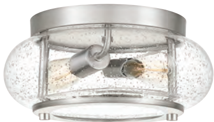
TRG1612BN 5.75" H x 12" W x 12" D 2 - 60W Medium Base (Not Included) ETL Listed Location: Damp
