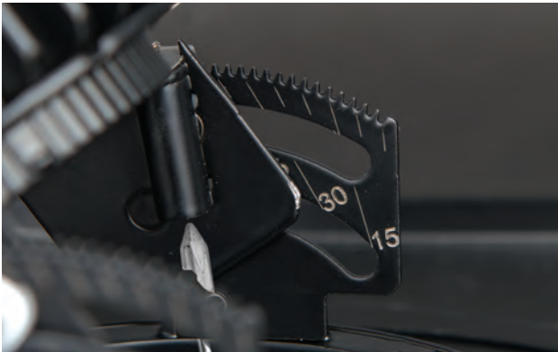
0-45° vertical lockable hot aiming
