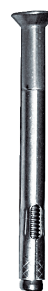
226 Stainless steel sleeve anchor Optional for all thresholds • An expansion anchor with a unique flat head machine screw all in one unit. • Easy installation. Place threshold in position and drill 1/4" dia. x 3 1/2" deep hole through countersunk hole in threshold. Drop the anchor in place and tighten with screwdriver.
